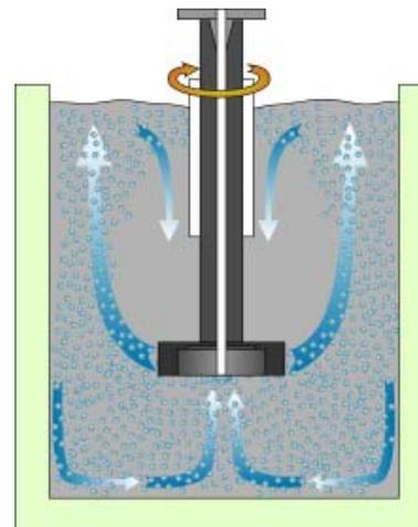
The above picture demonstrates the dramatic improvement in the dispersion of the inert gas bubbles and metal movement. Metal from the bottom of the ladle or well is drawn upward by the rotation of the rotor, eliminating untreated dead spots.
