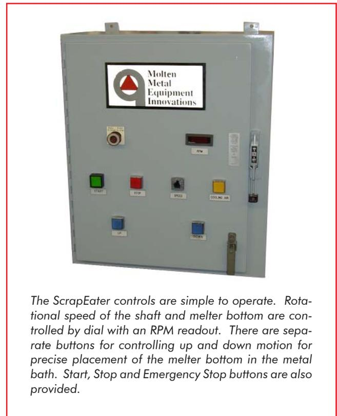
The ScrapEater controls are simple to operate. Rotational speed of the shaft and melter bottom are controlled by dial with an RPM readout. There are separate buttons for controlling up and down motion for precise placement of the melter bottom in the metal bath. Start, Stop and Emergency Stop buttons are also provided.
