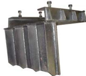
*The ScrapEater can be mounted on your floor or furnace sill. The above mounting plate is used when attaching the ScrapEater to the furnace sill. The mounting plate is welded onto the furnace sill. The ScrapEater can then be placed into the bracket using a forklift and bolted down. Removal is just as easy - simply unbolt and remove the ScrapEater with a forklift.*
