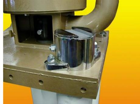
New post clamps are designed with a new flat on top to make it easier to assemble the MOLTAR. As the motor mount is lowered onto the posts, the flats allow the motor mount to rest on the posts as the clamp assemblies are tightened. Tighter tolerances ensure self-alignment of the entire pump.
