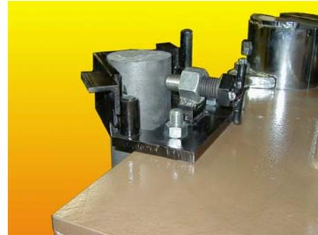
New injection tube clamp allows easy replacement of the injection tube. The 4" diameter tube is held securely in place with simple but secure locking device. Tube inserts vertically for easy installation - allows easier replacement in the molten metal without removing the pump. And because the tube is on the front of the pump, it helps reduce breakage from buildup between the tube and the shaft or posts.
