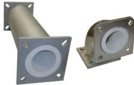
We also offer a complete range of refractory lined piping for use with the MIGHTY MITE Transfer Pump. We use large 2.5" diameter steel pipe with a 1.5" ID Liner to maximize flow while providing superior service life. We offer straights in any length up to 48" sections as well as elbows in nearly any angle required. As a result, we can provide you with piping to match your application requirements. Contact us for more information.
