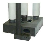
One of the advantages of the MMEI Circulation Pumps is that gas injection can be added to most models with our unique Foot & Tube method. The Foot & Tube is held in place by a clamp which bolts to the motor mount. Placed at the outlet of the pump, the gas is injected directly into the flow of metal for faster, more efficient metal treatment. It can be used to demag or degas. Contact us for more information.
