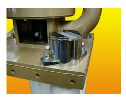
New post clamps are designed with a new flat on top to make it easier to assemble the MOLTAR. As the motor mount is lowered onto the posts, the flats allow the motor mount to rest on the posts as the clamp assemblies are tightened. Tighter tolerances ensure selfalignment of the entire pump.
