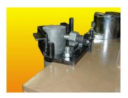
New injection tube clamp allows easy replacement of the injection tube. The 4" diameter tube is held securely in place with simple but secure locking device. Tube inserts vertically for easy installation - allows easier replacement in the molten metal without removing the pump. And because the tube is on the front of the pump, it helps reduce breakage from buildup between the tube and the shaft or posts.
