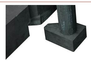
The THOR features an advanced Foot & Tube gas injection method. The gas is injected into the bottom of the outlet of the base ensuring maximum shearing. The flow of metal actually draws the gas into the flow, reducing leakage and improving mixing for faster metal treatment
