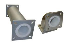
We also offer a complete range of refractory lined piping for use with the MIGHTY MITE Transfer Pump. We use large 2.5" diameter steel pipe with a 1.5" ID Liner to maximize flow while providing superior service life. We offer straights in any length up to 48" sections as well as elbows in nearly any angle required. As a result, we can provide you with piping to match your application requirements. Contact us for more information.
